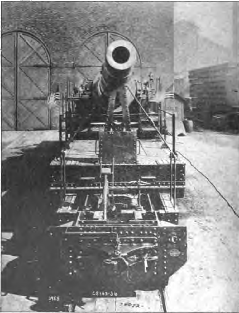
12-INCH, 35-CALIBER AMERICAN GUN ON BATIGNOLLES MOUNT.
